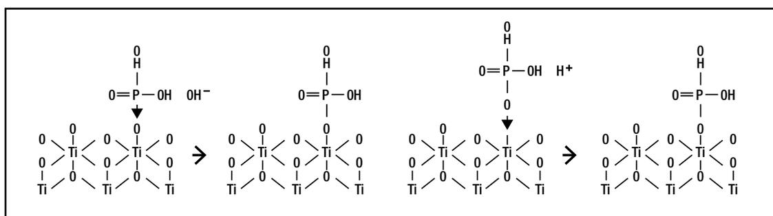
**Figure 5.** Theoretical scheme of phosphoric acid-titanium oxide structure, inferred from studies of electron spectroscopy.<sup>13</sup>
