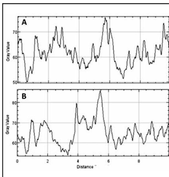
**Figure 4.** The graphs present the profiles of the average gray levels outline of the images of implants surfaces, previously converted to gray images of 16 bits. The ordinate shows the average gray level of the 720 pixels for each one of the 969 pixels of the width of the images. **A.** Implants anodized in phosphoric acid 2M; **B.** Anodized in phosphoric acid 2M+NaF 0.2M.
